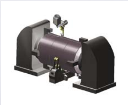
Joining of shell sections using roller beds or a head and tailstock positioner. External submerged-arc welding performed by a column and boom station.
