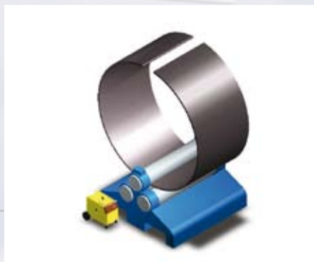
Rolling, forming and tack welding of the shell
