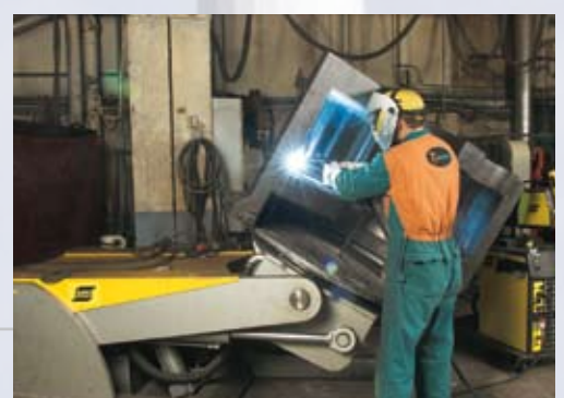
Production of sub components (gear box housing), using an ESAB positioner and manual welding equipment.
