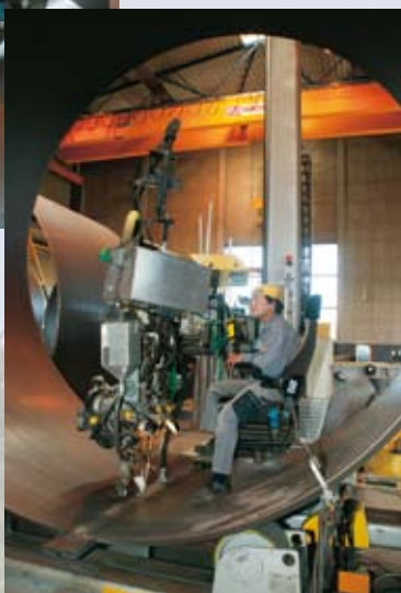
Internal longitudinal submerged-arc welding using a column and boom
