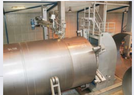
Joining of shell sections using roller beds or a head and tailstock positioner. External submerged-arc welding performed by a column and boom station.
