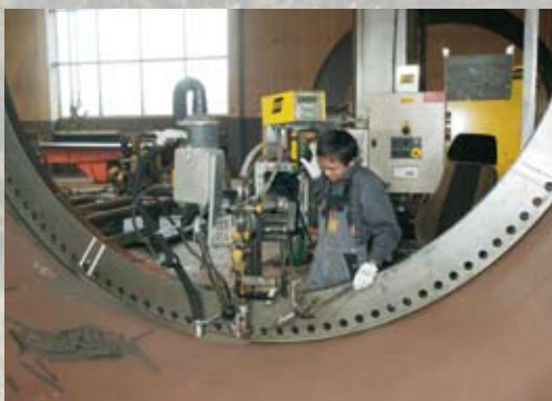
Manual MAG welding or submerged-arc welding of flanges and supports
