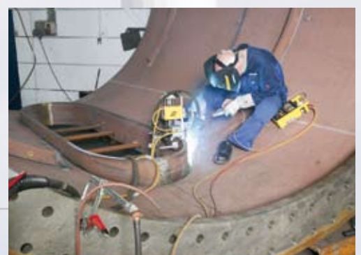
Automatic welding of door frame using an ESAB Frametrac. A MIG/MAG welding tractor specially designed for travelling along a door frame.
