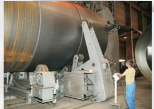
Hydraulic forming of shell sections when tack welding.
