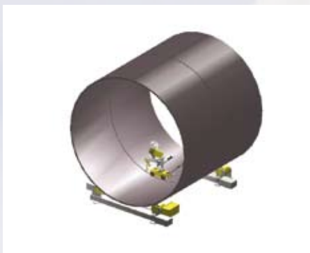
Joining of shell sections using an ESAB Tripletrac. A tractor unit specially designed for internal welding.
