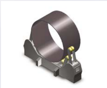
Hydraulic forming of shell sections when tack welding.
