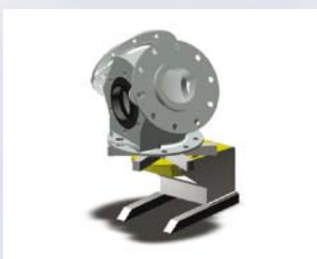
Production of sub components (gear box housing), using an ESAB positioner and manual welding equipment.
