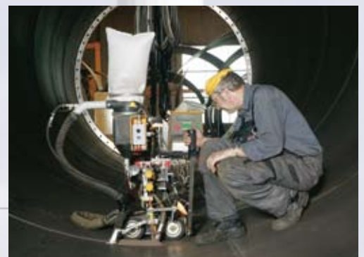
Joining of shell sections using an ESAB Tripletrac. A tractor unit specially designed for internal welding.
